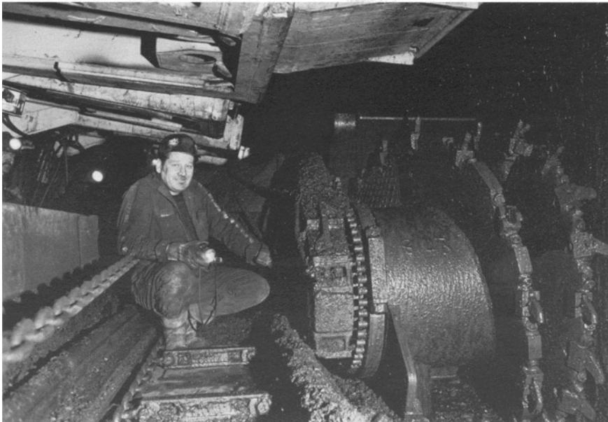
Hydraulic roof shields and longwall face shearer in a modern coal mine of the Sydney coalfield. (Owen Fitzgerald photograph).
